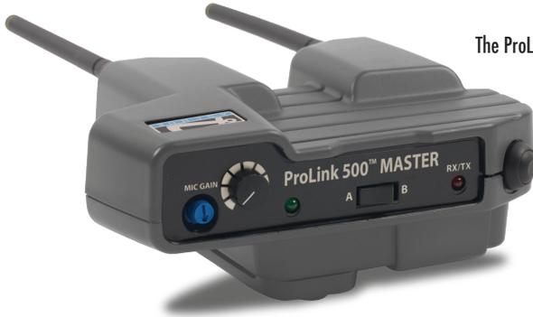
The ProLink 500 is a digital wireless intercom system that allows full duplex communication between four users simultaneously with the option of unlimited number of listen only belt packs. The transmitter and receiver operate utilizing the FCC license free 902 - 928 MHz range for the U.S. without the need for a base station. The ProLink 500 has the capability to transmit
